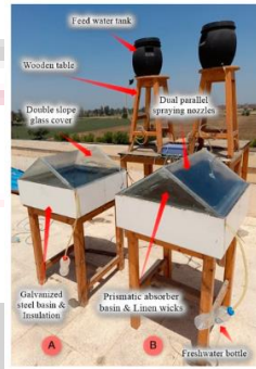
Figure 3: Photographic view of the test-rig of TDSSD A and DSSD-WPB&DPSN B [32]
